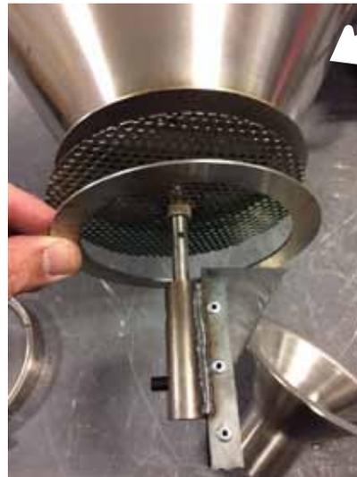
Brush adjustment may be necessary as brush wears. To adjust the brush, loosen the 4-1/4" motor mount bracket bolts with 7/16" wrench. Apply downward pressure on top of the motor until there is proper brush contact with the screen. Bristles should lean back slightly when brush rotates.
